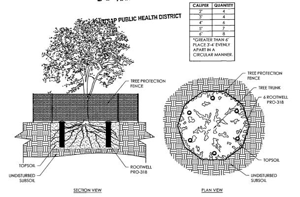
1. EXISTING TREES REQUIRE THE ROOTWELL TO BE PLACED APPROXIMATELY 2.5' TO 4' FROM THE TRUNK, OR ON LARGE TREES AS CLOSE AS POSSIBLE. TREE ROOTS ARE NOT AT THE DRIP LINE, BUT ARE MUCH CLOSER TO THE TRUNK WHEN TREES ARE IN STRESS, IN DECLINE, OR IN COMPACTED SOILS.
